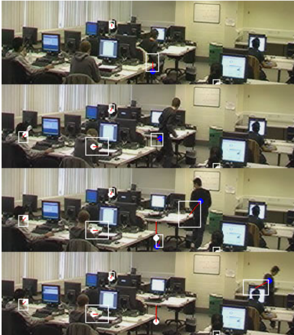
Colour Plate C: Example of regioned and free object tracking. Notice as the student gets out of the chair, he moves it backward abruptly, and an additional free object is falsely assigned to it. Also note how, in the final frame, the student's bounding box passes through another regioned area without any ill effect
